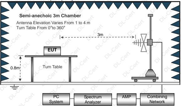
(C) Radiated Emission Test-Up Frequency Above 1GHz
