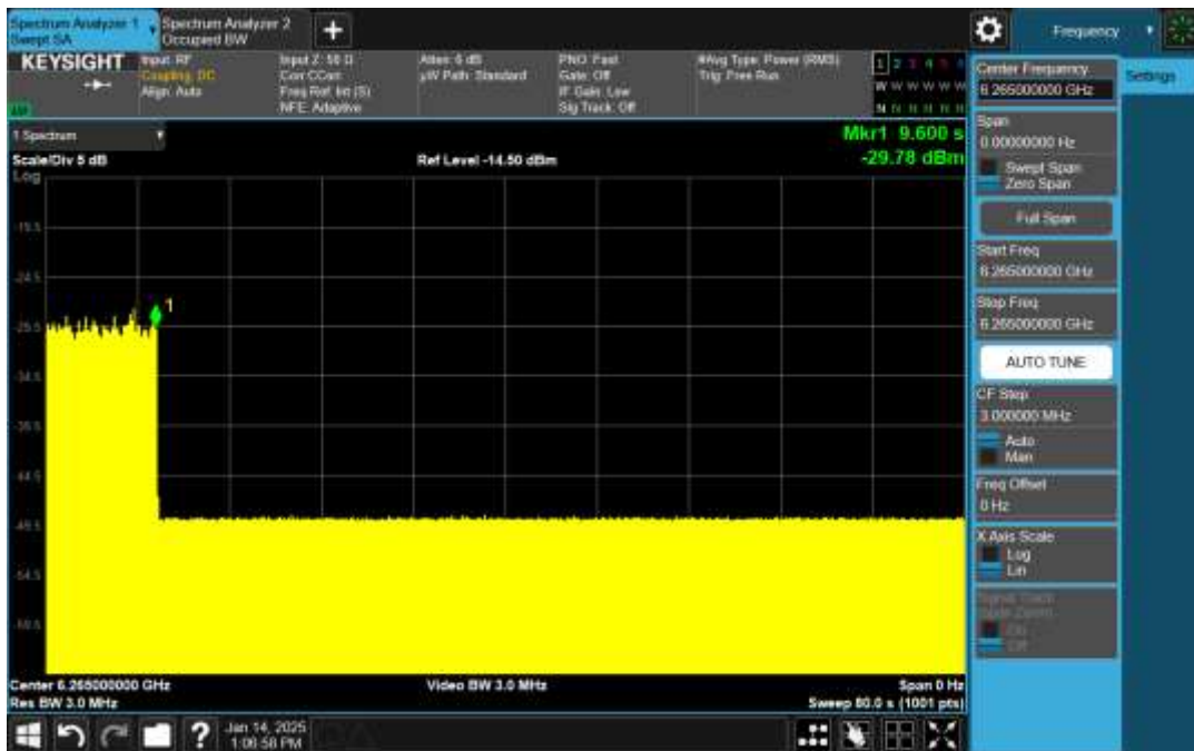
Plot 12: AWGN Signal Detection 320MHz
