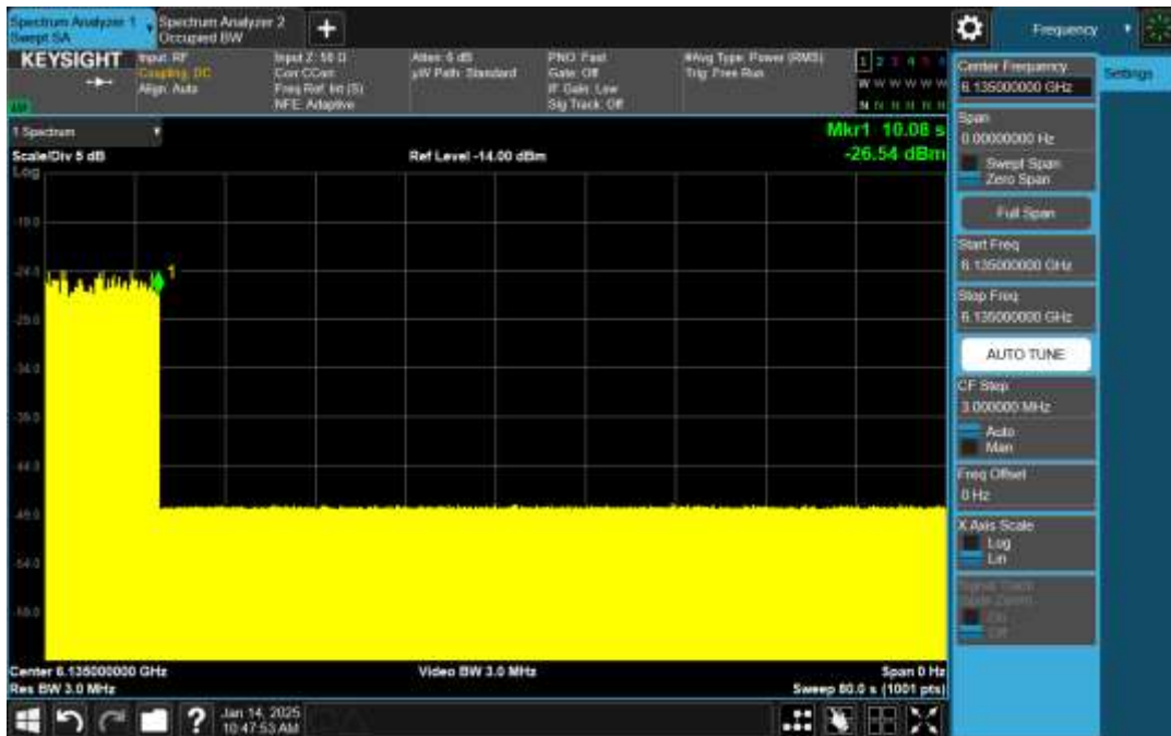
Plot 3: AWGN Signal Detection 20MHz
