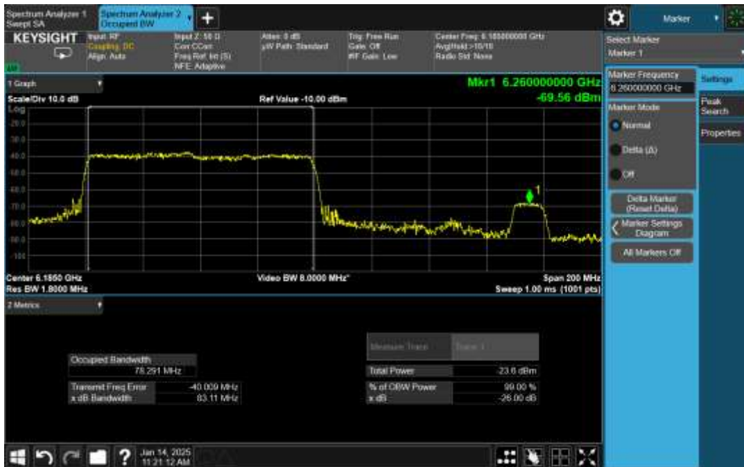
Plot 5: EUT 160MHz Bandwidth Reduction
