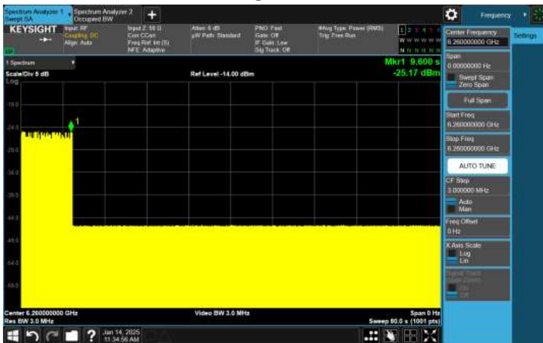
Plot 8: AWGN Signal Detection 160MHz
