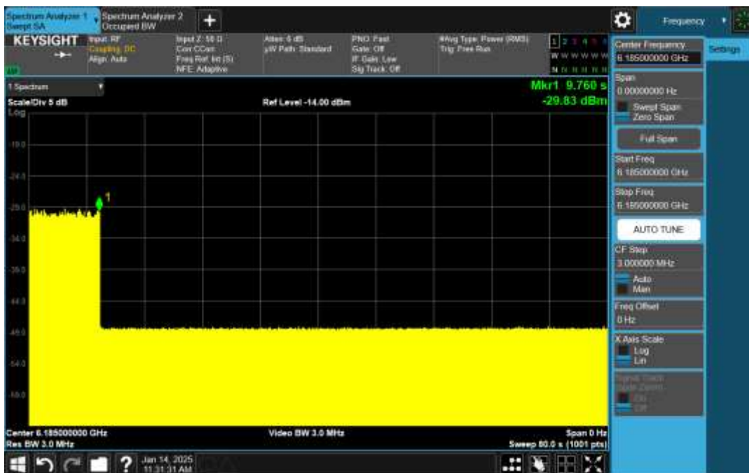
Plot 7: AWGN Signal Detection 160MHz
