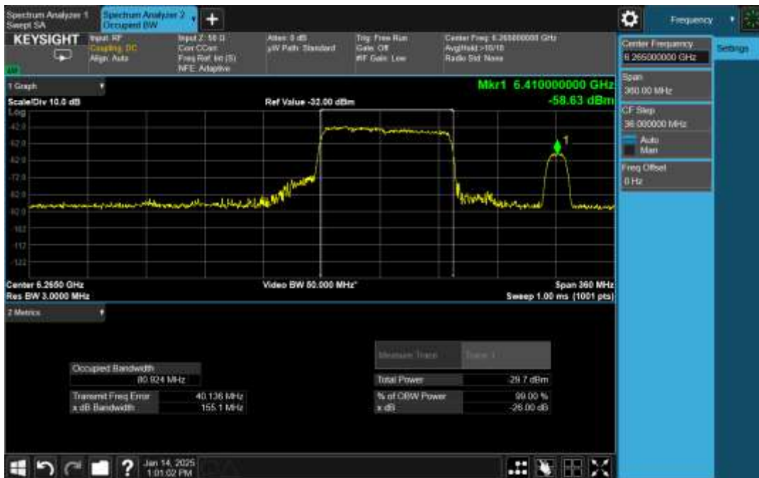
Plot 10: EUT 320MHz Bandwidth Reduction
