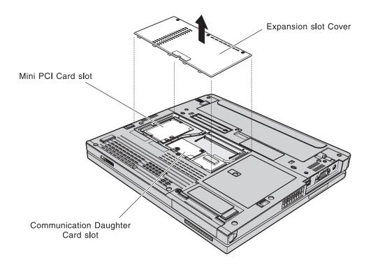
**Attention:** The ThinkPad X41 Tablet Series computer contains an authentication mechanism You can install or remove each wireless feature by yourself. If you install an unauthorized wireless adapter that is not approved for use in the ThinkPad X41 Tablet Series computer, the computer will not start, but only displays an error message and emits beeps.
