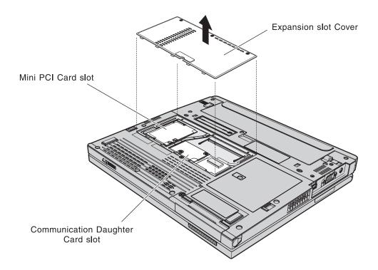
**Attention:** The ThinkPad X41 Tablet Series computer contains an authentication mechanism If you install an unauthorized wireless LAN Mini-PCI Card or RF CDC module that is not approved for use in the ThinkPad X41 Tablet Series computer, the computer will not start, but only displays an error message and emits beeps.
