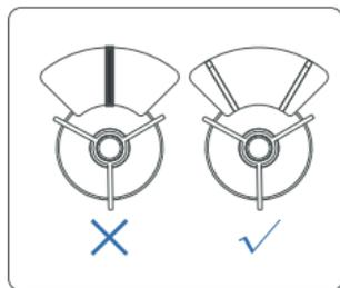
● Pay attention to the direction of the impeller; the impeller should not be placed in the center.
