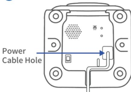
● Check the bottom of the device and plug in the USB cable.
