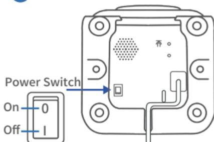
● Turn on the power switch at the bottom of the feeder.
