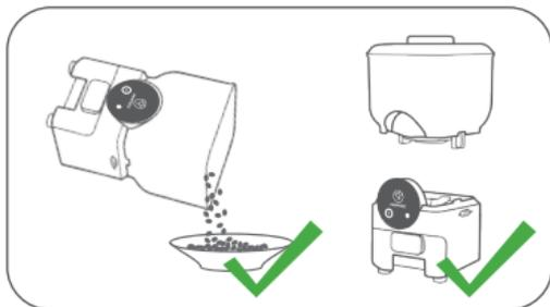
When disassembling the food tank, please pour out all the food before disassembling it to avoid spilling.
