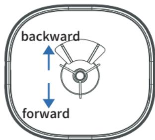
● When installing the food impeller: Please pay attention to the impeller direction.
