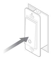
Attach the wallplate and turn on the circuit breaker. Then the wiring is finished.
