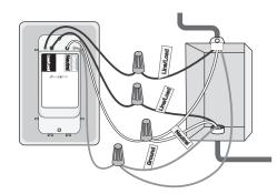
Line up the switch with the mounting holes. Secure it with screws.
