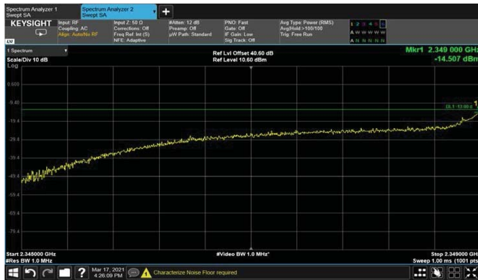
Figure 159. —2345.0MHz -2349.0MHz -64QAM-4G
