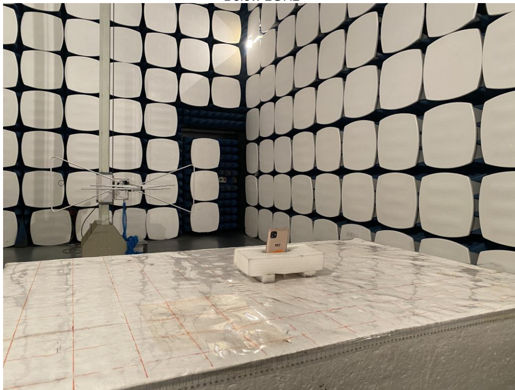
Radiated Spurious Emission Below 1GHz
