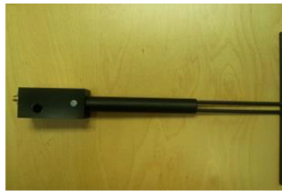
Figure 1 – MVG COMOSAR Validation Dipole
