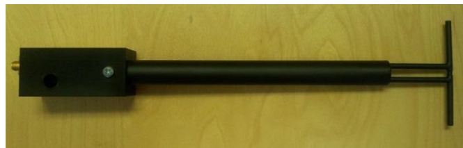
Figure 1 – MVG COMOSAR Validation Dipole
