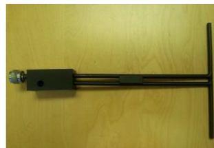
Figure 1 – MVG COMOSAR Validation Dipole
