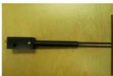
Figure 1 – MVG COMOSAR Validation Dipole
