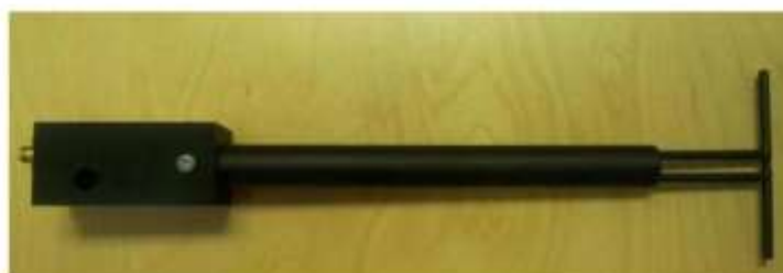
Figure 1 – MVG COMOSAR Validation Dipole
