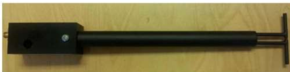
Figure 1 – MVG COMOSAR Validation Dipole
