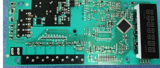
2. The new mother board is the same input and output to the original except for PCB layout and some components differences.
