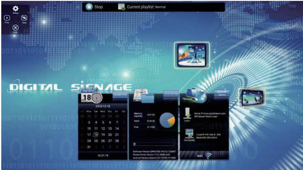
The middle of the top displays the current playing status, the bottom from the left to right are time, date and local storage (including apk version, firmware version, local storage). The working mode is LAN by default.
