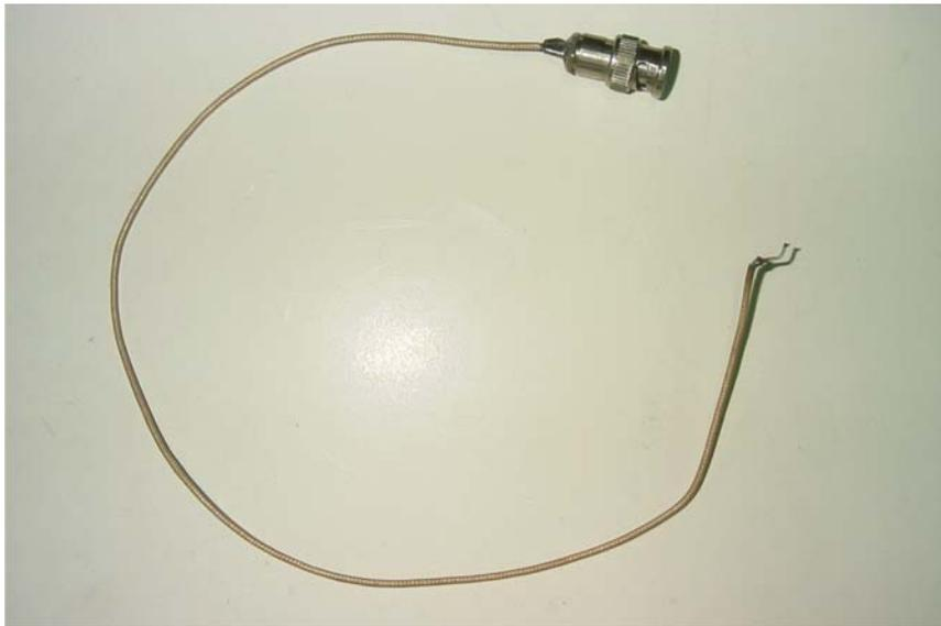
Figure 2.2. RF test cable
