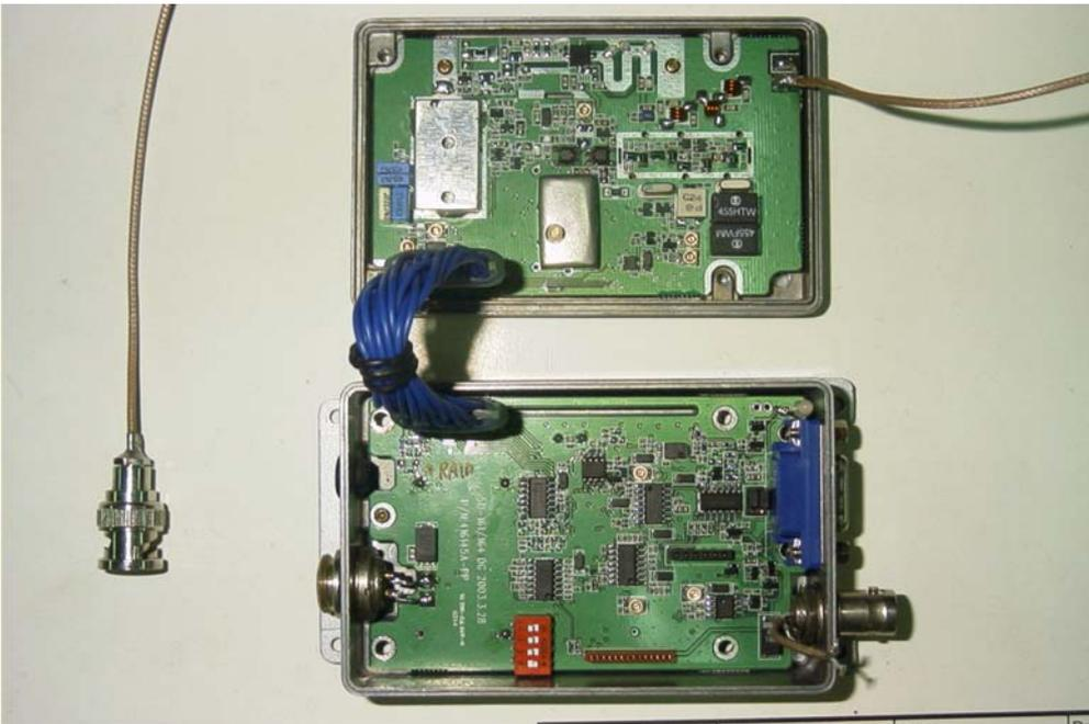
Figure 2.3. Connecting RF board to Digital board
