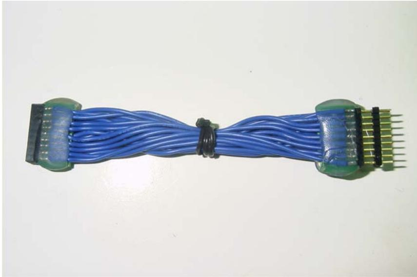
Figure 1.1. Flexible PCB Extender
