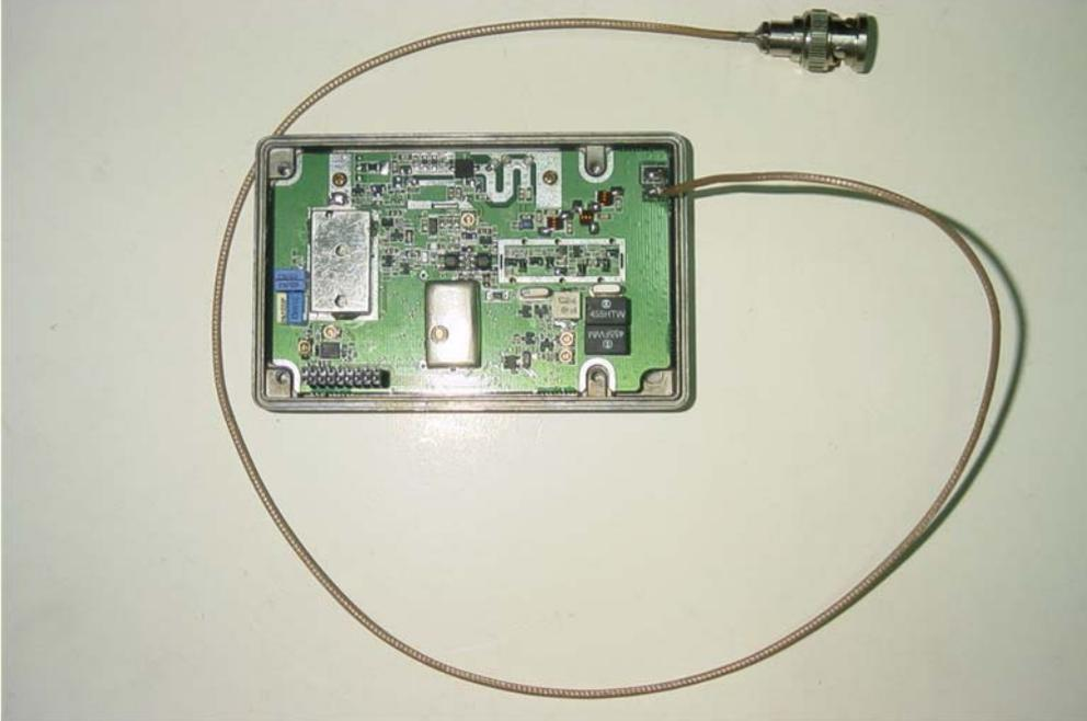
Figure 2.2. Soldering RF test cable to RF board
