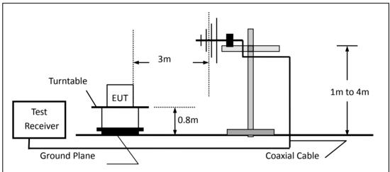
(c) For radiated emissions above 1000MHz
