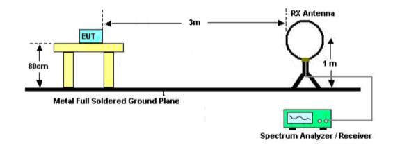
(B) Radiated Emission Test-Up Frequency 30MHz~1GHz
