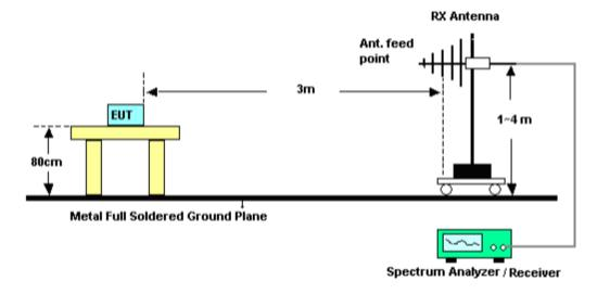
(C) Radiated Emission Test-Up Frequency Above 1GHz
