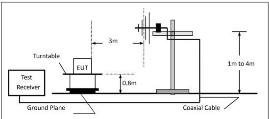
(c) For radiated emissions above 1000MHz
