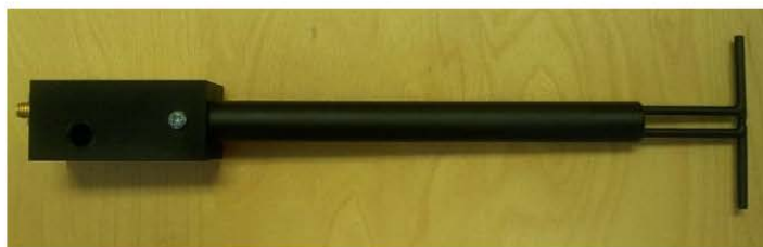
Figure 1 – MVG COMOSAR Validation Dipole
