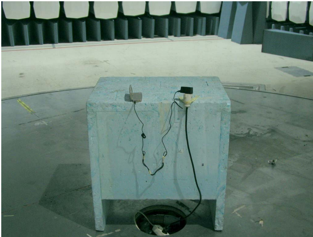
Photograph 1. Radiated spurious emissions test setup
