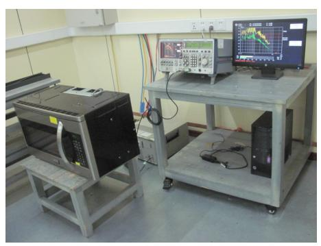
Radiated Emission Test Set-up (30 -1,000MHz):
