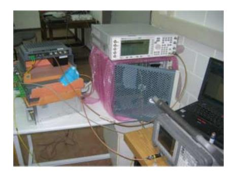
Photograph No.2 Spurious emissions measurements at RF antenna connector test setup
