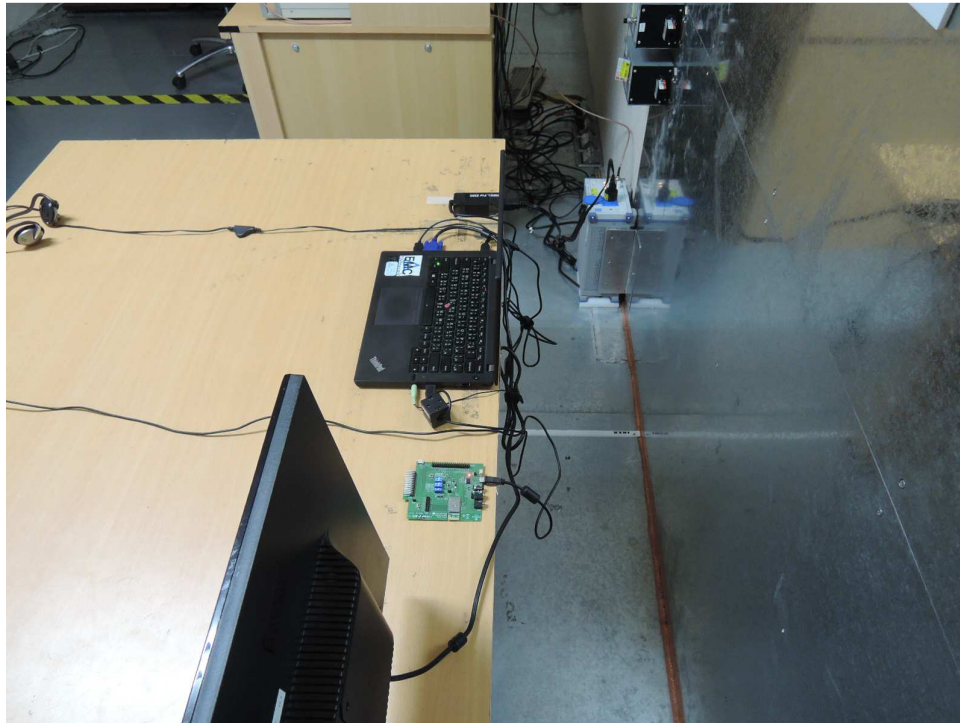
Photograph 5: Set-up for for Mains Conducted testing Back
