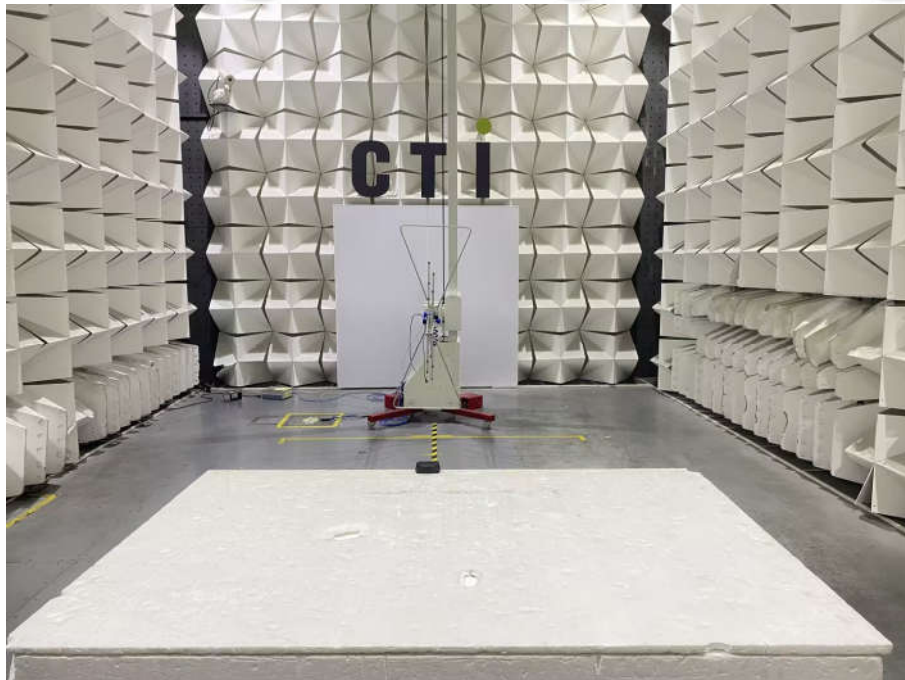
Radiated spurious emission Test Setup-1(Below 1GHz)
