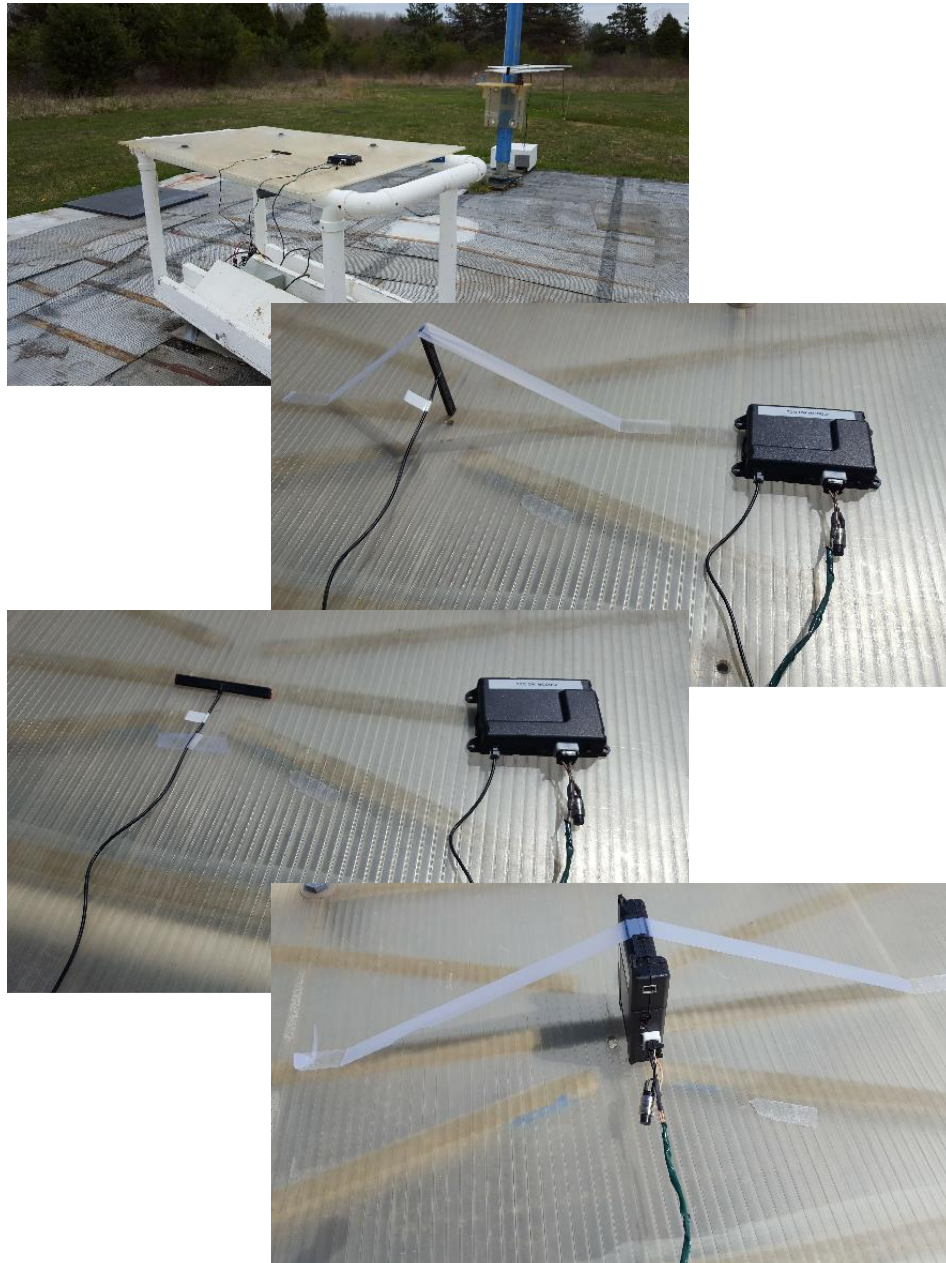
Figure 4: Radiated Emissions Test Setup Photograph(s).
