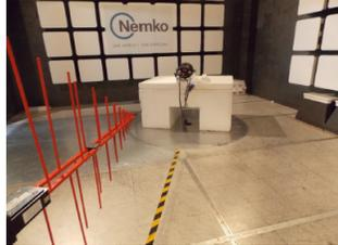
Figure 8.1-3: Radiated emissions setup photo - below 1 GHz
