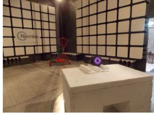
Figure 8.1-2: Radiated emissions setup photo - below 1 GHz
