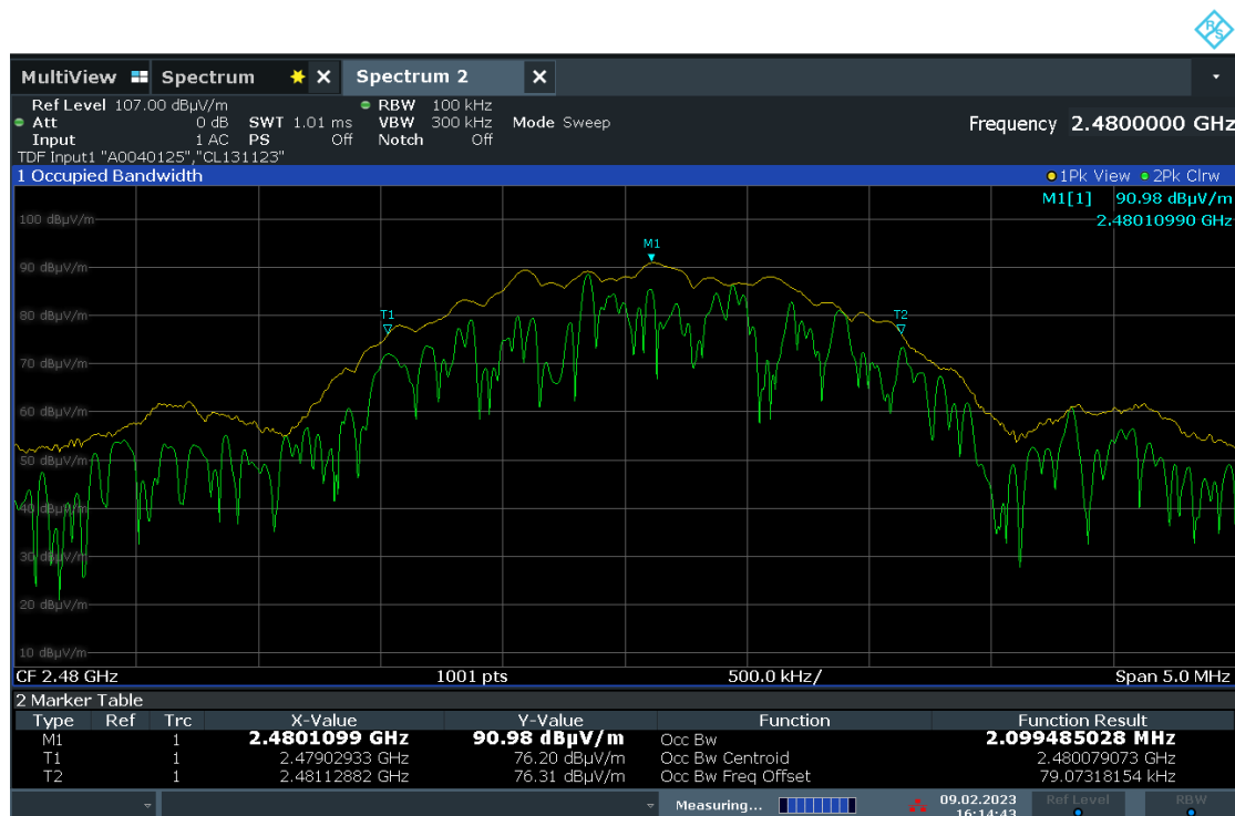
Graph 6-33: Occupied bandwidth, 2480 MHz
