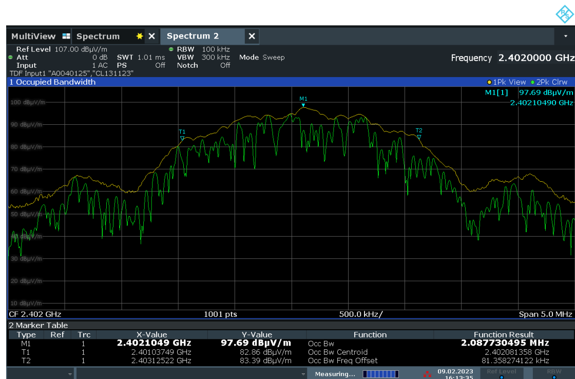
Graph 6-31: Occupied bandwidth, 2402 MHz
