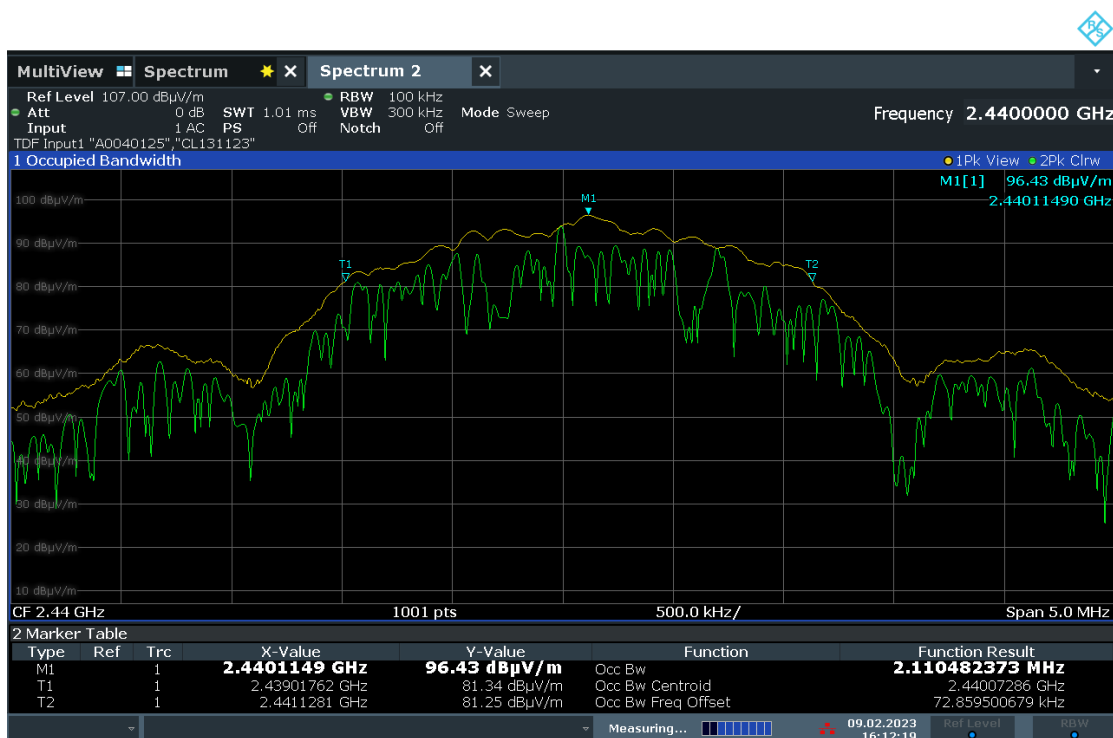
Graph 6-32: Occupied bandwidth, 2440 MHz
