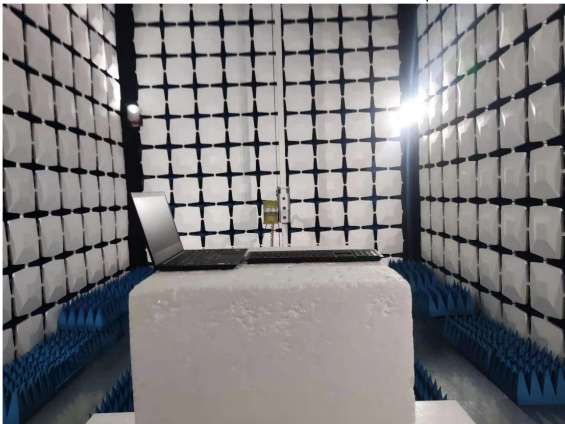
Above 1GHz for radiated emission test setup
