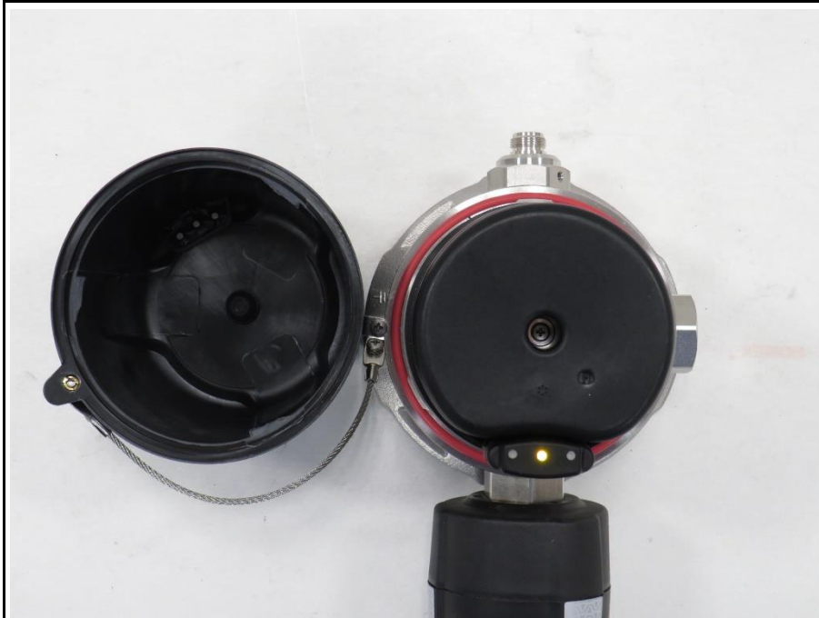
EUT BATTERY POWERED WITH OPEN COVER AND BATTERY
