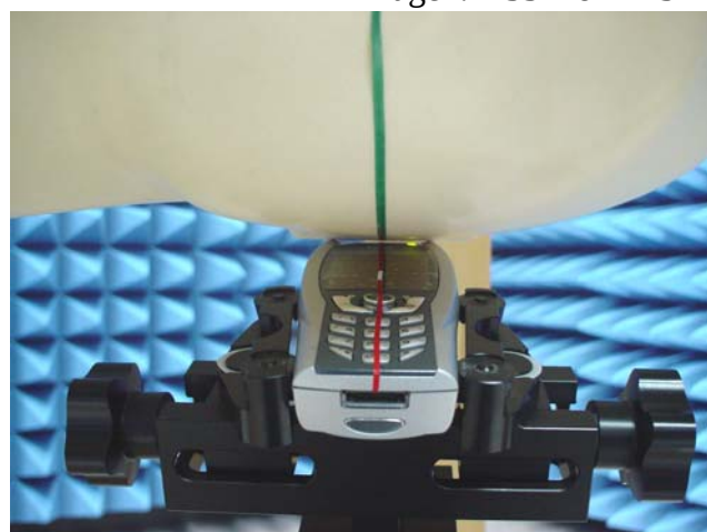
Fig.7 Left Head Section / Ear-Tilt Position(15°)
