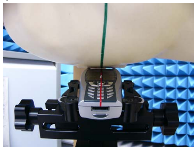
Fig.4 Right Head Section / Cheek-Touch Position
