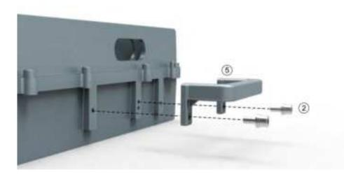
2. Attach and fasten the Bracket I to the left side of HPRU with screws M6×14 using T5 Wrench.
