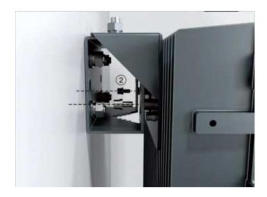
8. Connect and lock the power cable at the HPRU rear side.
