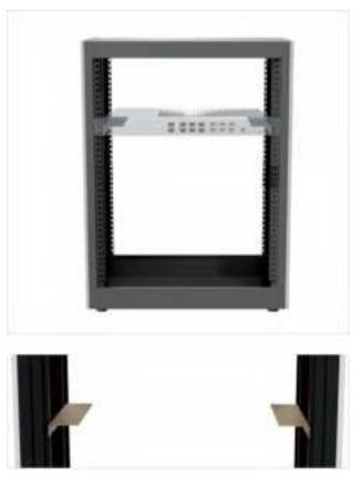
3. Place the EU in the rack and secure the EU using 2 screws M6×16 on both sides and the Phillips screwdriver.
