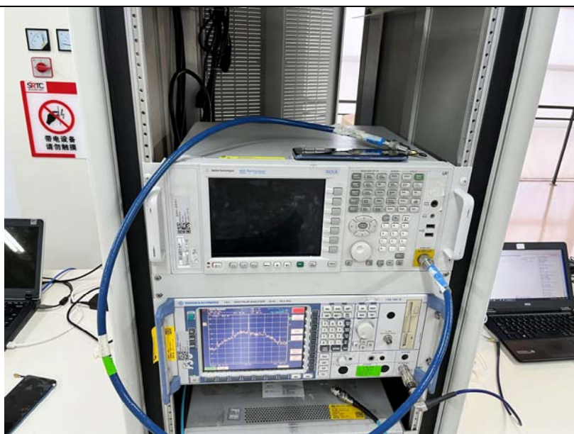
RF Conducted Test setup (BT/WIFI)
