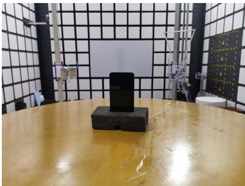
Spurious Radiated Emissions Test setup
