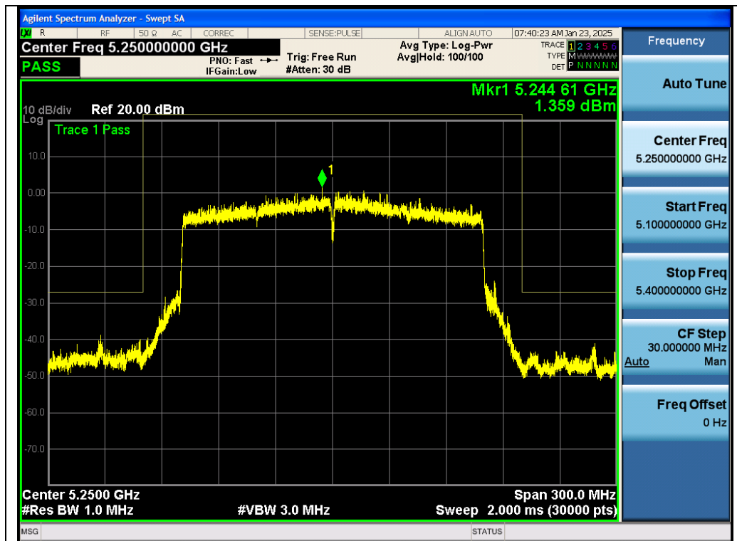
Test_Graph_802.11ax160_Chain A_5250_MCS0_Frequency Band 3
