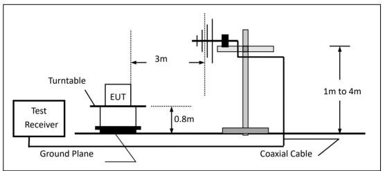
(c) For radiated emissions above 1000MHz
