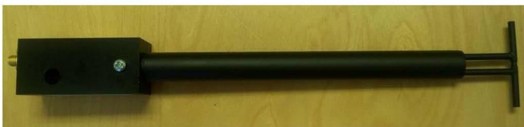
Figure 1 – MVG COMOSAR Validation Dipole
