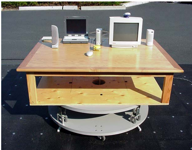
Photograph E-3 - Front of Radiated Emission Configuration
