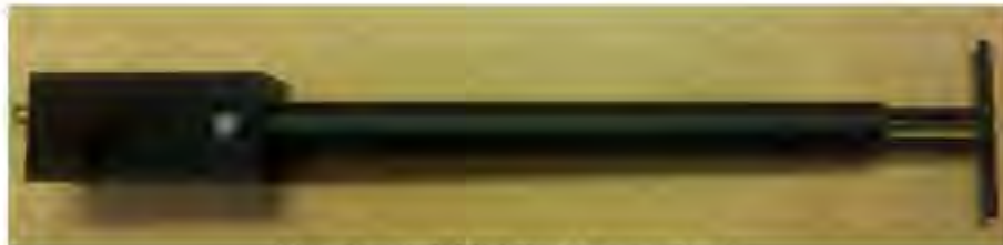
Figure 1 – MVG COMOSAR Validation Dipole
