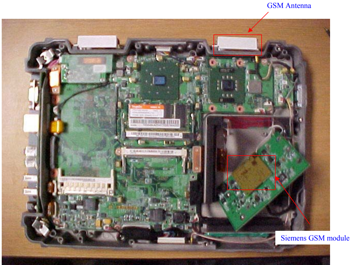
EUT – Internal view showing GSM module
