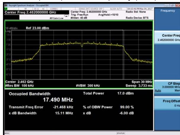
802.11n(HT20), Carrier frequency (MHz): 2462
