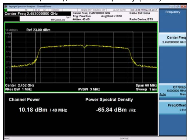
802.11n(HT40), Carrier frequency (MHz):2452
