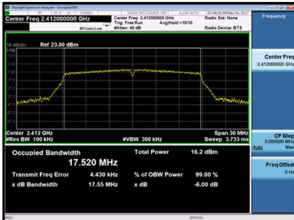
802.11n(HT20), Carrier frequency (MHz): 2437
