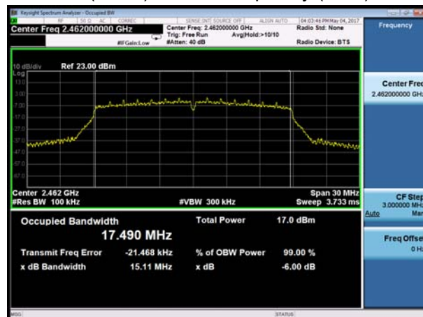
802.11n(HT20), Carrier frequency (MHz): 2462
