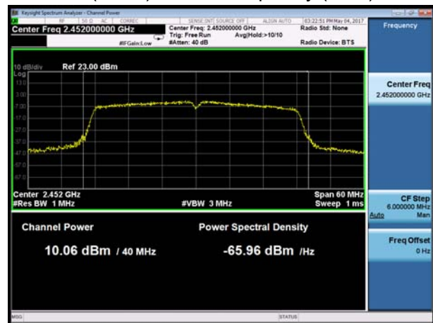
802.11n(HT40), Carrier frequency (MHz):2452
