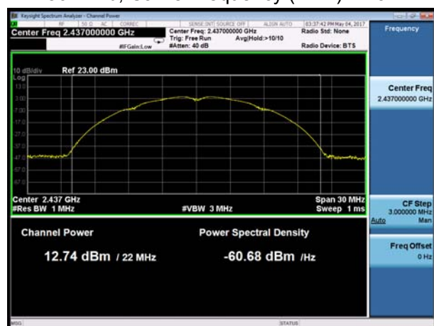
802.11b, Carrier frequency (MHz): 2437
