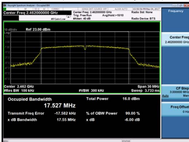
802.11n(HT20), Carrier frequency (MHz): 2462
