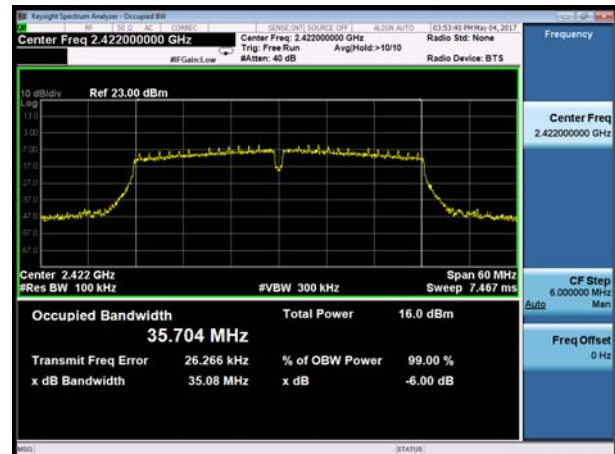
802.11n(HT40), Carrier frequency (MHz): 2437
