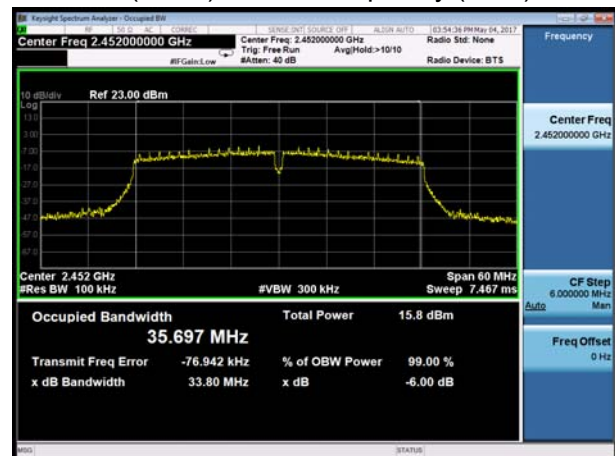
802.11n(HT40), Carrier frequency (MHz): 2452
