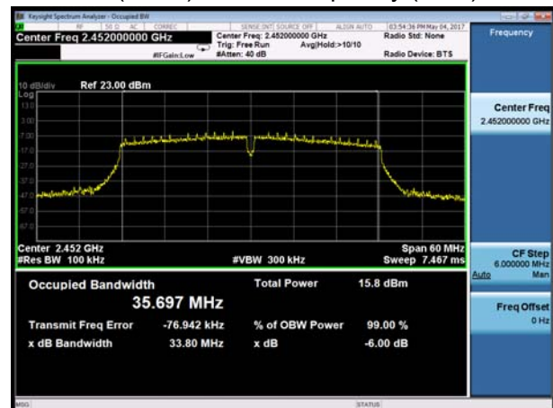
802.11n(HT40), Carrier frequency (MHz): 2452
