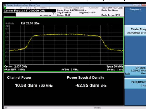
802.11n(HT20), Carrier frequency (MHz): 2437
