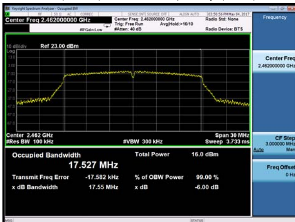
802.11n(HT20), Carrier frequency (MHz): 2462
