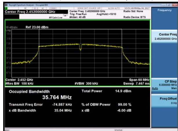
802.11n(HT40), Carrier frequency (MHz): 2452
