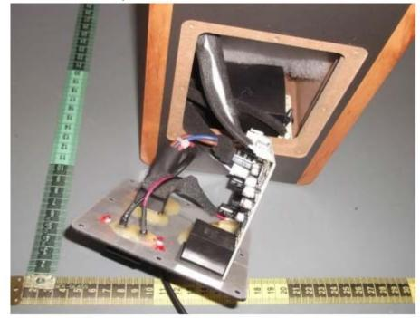
M/N: EDF100035: the power board is mounted on the rear panel and the PCB motherboard is mounted horizontally
