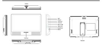
OPEN(  $\blacksquare$ ): Press it to open the unit and put the disc on the loading tray.
