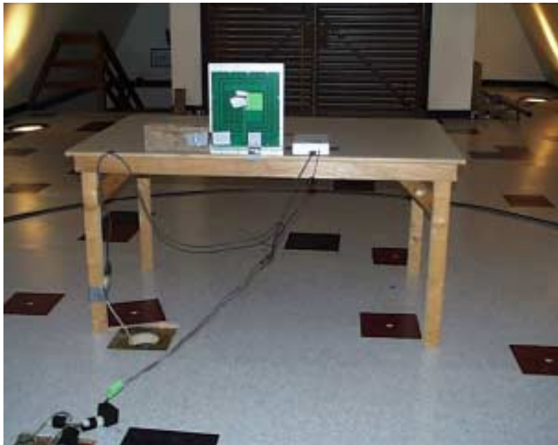
Photo 4 – Radiated Emissions Test Setup – Rear View
