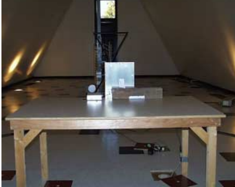
Photo 3 – Radiated Emissions Test Setup – Front View
