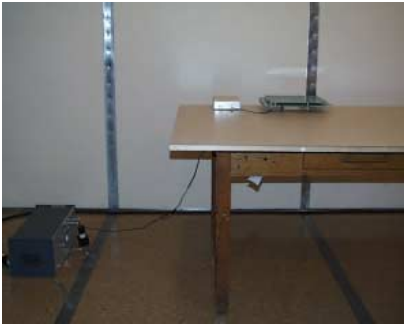
Photo 6 – Conducted Emissions Test Setup – Front View
