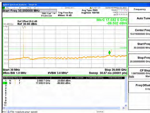
B7-30M-20G / 20MHz / High CH / QPSK
