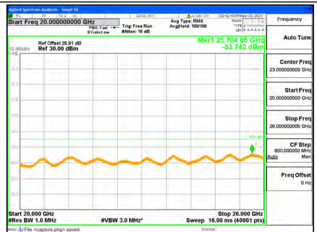
B7-20G-26G / 5MHz / High CH / QPSK
