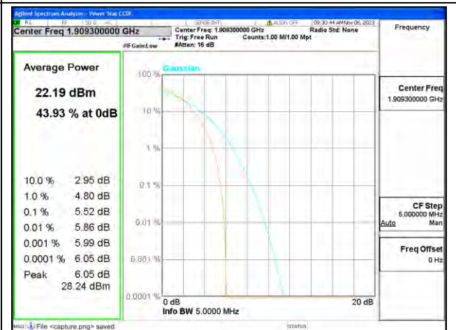
B2 / 1.4MHz / High CH / 16QAM
