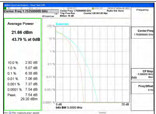
B4 / 5MHz / High CH / 16QAM
