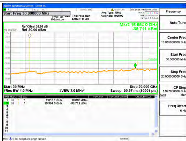
B38-30M-20G / 5MHz / High CH / QPSK
