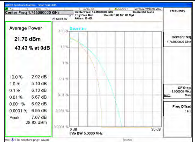
B66 / 3MHz / Mid CH / 16QAM
