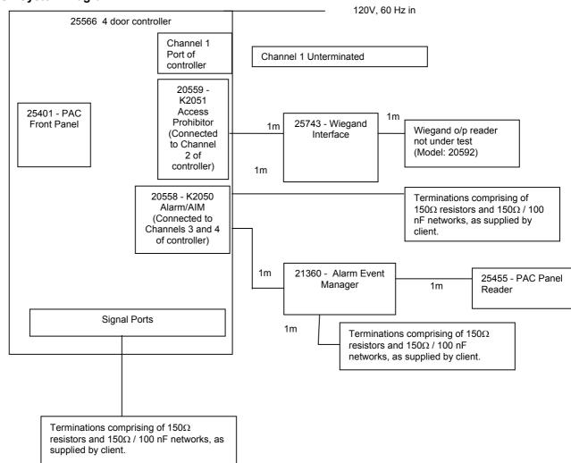
NOTE: When testing PAC part 25401 to sec. 15.209, only the signal ports on the diagram above were terminated. Ports 1,2,3 and 4 were unterminated (i.e. no other PAC items were connected to the controller)
