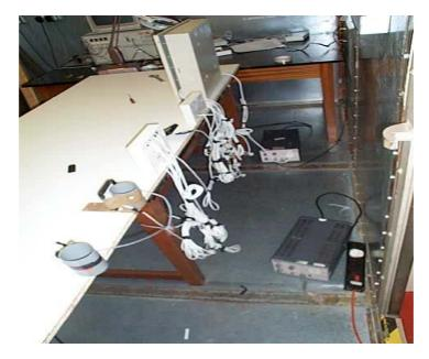
Note: The test was performed with a 40cm separation distance between the EUT and the vertical ground plane. The table was moved away from the vertical ground plane to allow a clearer photograph of EUT and cable setup to be taken.
