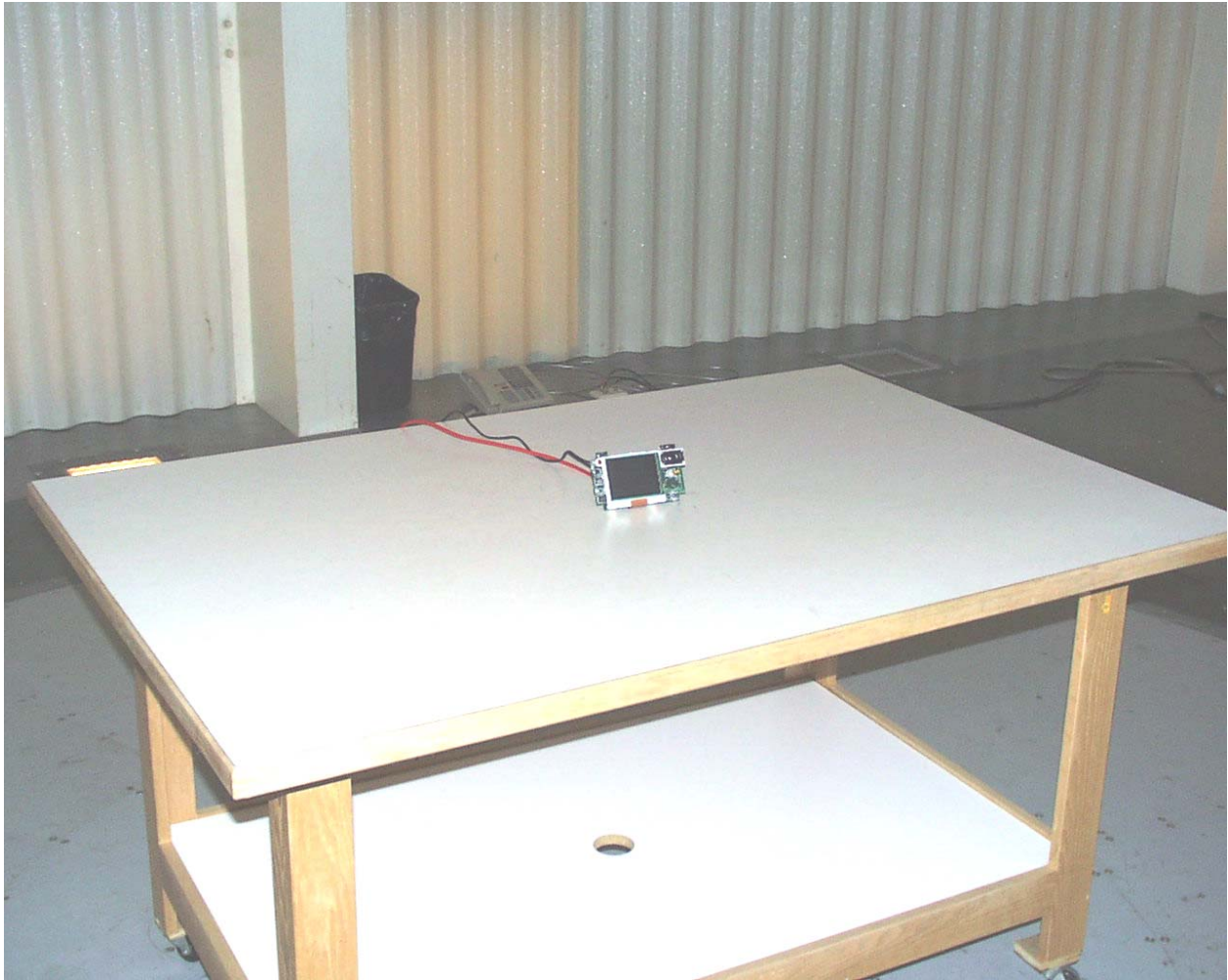
Photograph 1 - Front View Radiated Disturbance Worst Case Configuration
