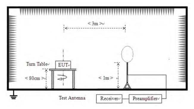
2) For radiated emissions from 30MHz to1GHz
