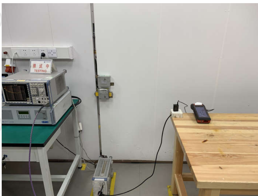
Conducted Emissions Test Setup
