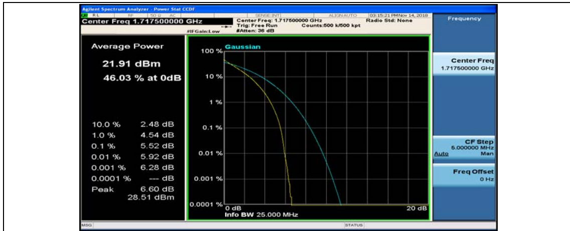
(Channel Bandwidth:15 MHz)_MCH_QPSK_1RB#0
