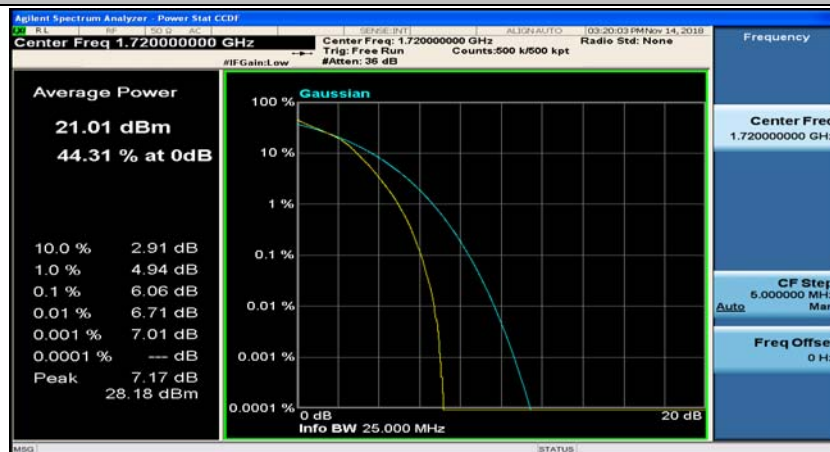
(Channel Bandwidth:20 MHz)_LCH_16QAM_100RB#0
