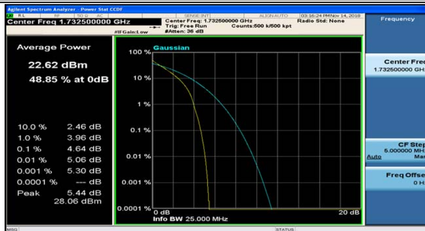
(Channel Bandwidth:15 MHz)_MCH_QPSK_37RB#38
