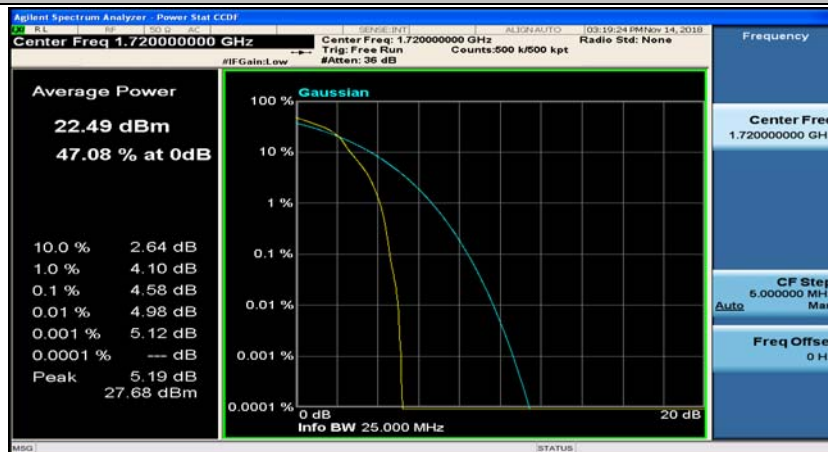
(Channel Bandwidth:20 MHz)_LCH_16QAM_50RB#0
