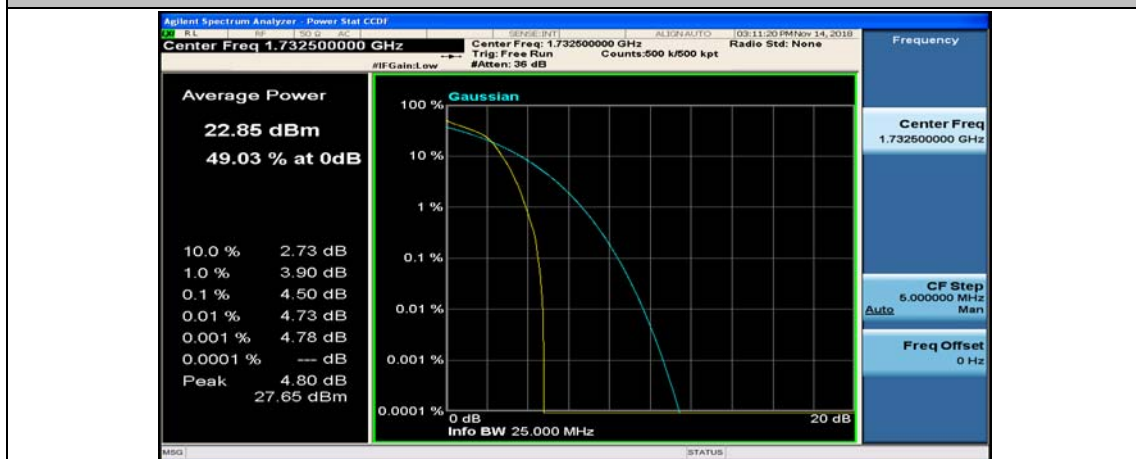
Channel Bandwidth: 10 MHz_MCH_16QAM_1RB#49
