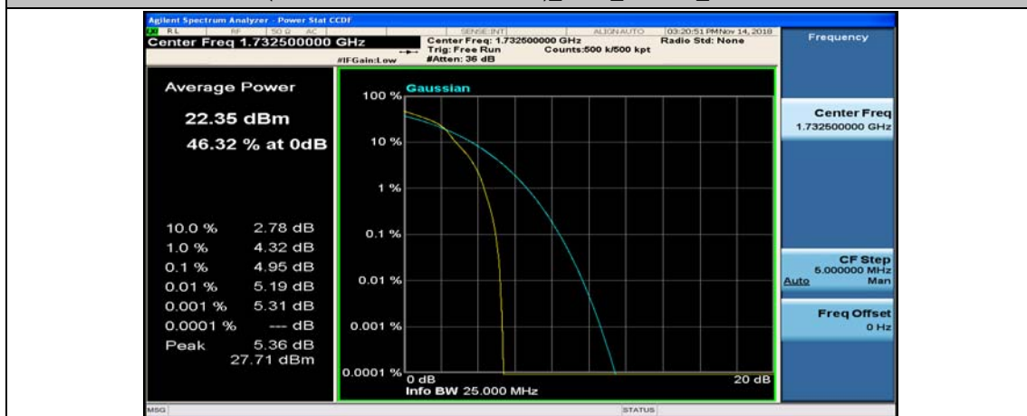
(Channel Bandwidth:20 MHz)_MCH_16QAM_1RB#49
