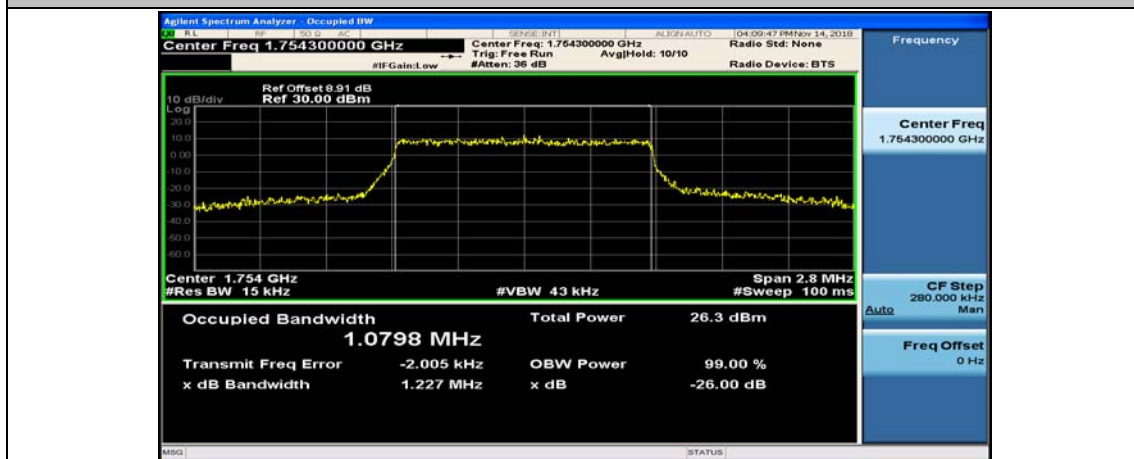
(Channel Bandwidth: 1.4 MHz)_HCH_QPSK_6RB#0
