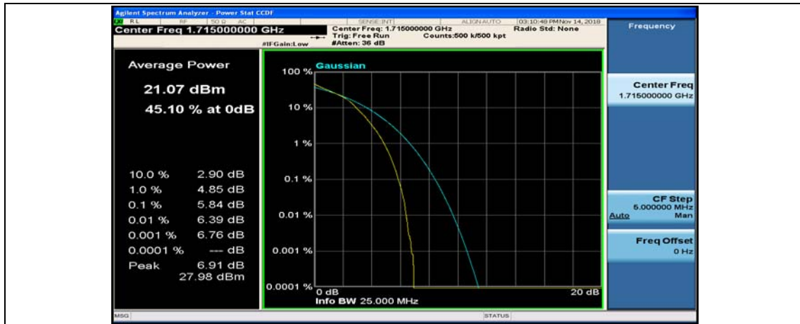
Channel Bandwidth: 10 MHz_MCH_16QAM_1RB#0
