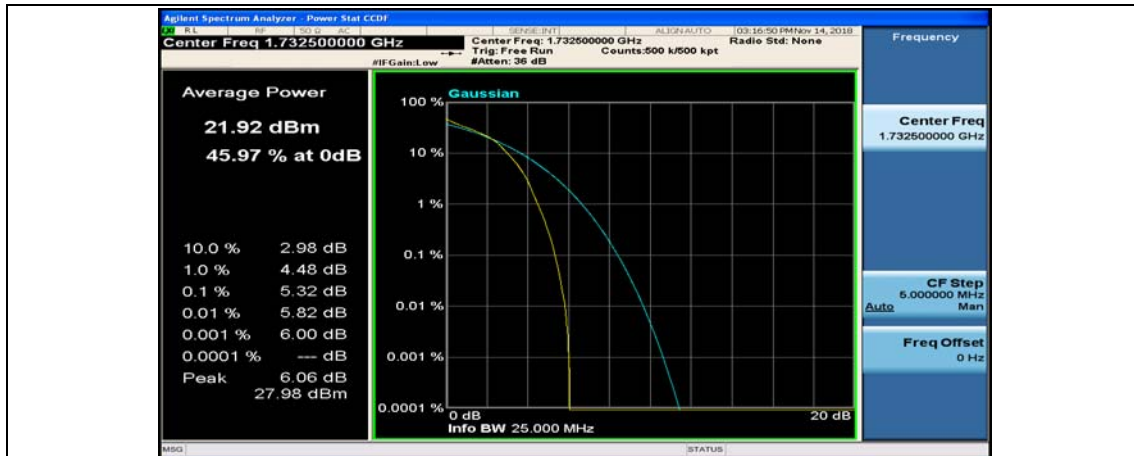
(Channel Bandwidth:15 MHz)_MCH_16QAM_75RB#0
