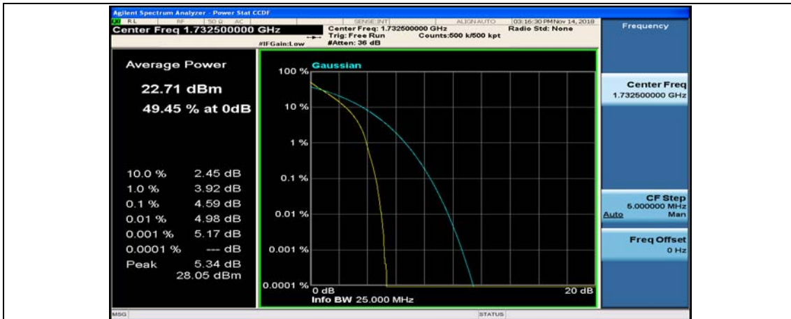
(Channel Bandwidth:15 MHz)_MCH_QPSK_75RB#0
