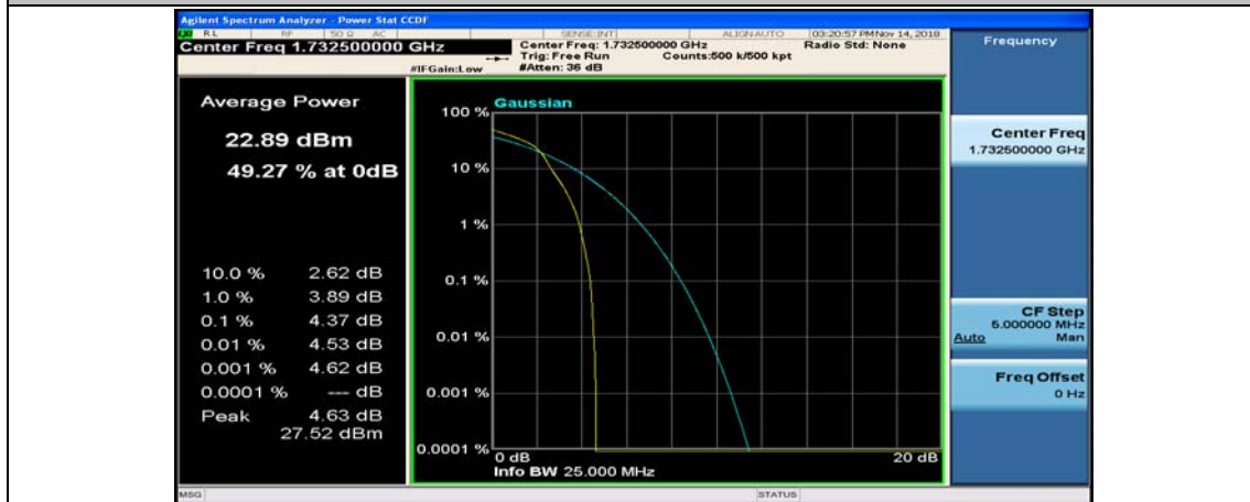
(Channel Bandwidth:20 MHz)_MCH_16QAM_1RB#99
