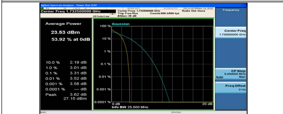
Channel Bandwidth: 10 MHz_MCH_QPSK_1RB#49
