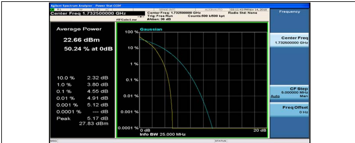
Channel Bandwidth: 10 MHz_MCH_QPSK_50RB#0
