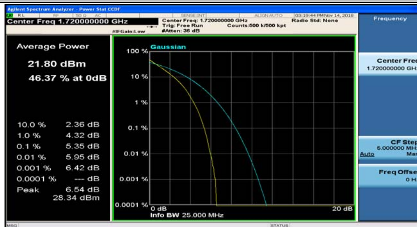
(Channel Bandwidth:20 MHz)_LCH_QPSK_100RB#0
