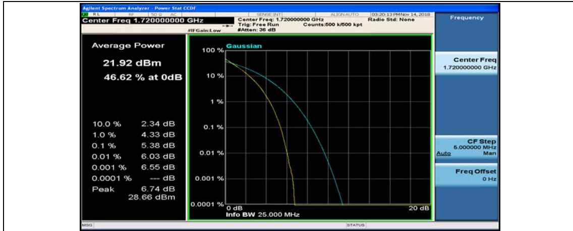
(Channel Bandwidth:20 MHz)_MCH_QPSK_1RB#0
