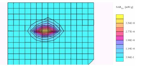
Validation Dipole SAR 1900 MHz (Ambient Temp = 23 C, Liquid Temp = 21 C) SAM Phantom; Flat Section; Position: (90°,90°); Frequency: 1900 MHz Probe: ET3DV6 - SN1604; ConvF(4.90,4.90,4.90); Crest factor: 1.0; Body 1900 MHz:  $\sigma = 1.53$  mho/m  $\epsilon_r = 55.5 \ \rho = 1.00$  g/cm<sup>3</sup> Cube 5x5x7: SAR (1g): 3.40 mW/g, SAR (10g): 1.85 mW/g, (Worst-case extrapolation) Coarse: Dx = 12.0, Dy = 12.0, Dz = 10.0 Powerdrift: -0.00 dB
