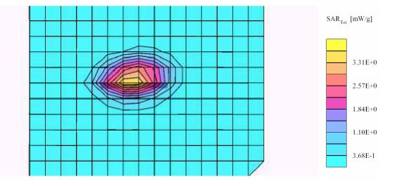
Validation Dipole SAR 1900 MHz (Ambient Temp = 23 C, Liquid Temp = 21 C) SAM Phantom; Flat Section; Position: (90°,90°); Frequency: 1900 MHz Probe: ET3DV6 - SN1604; ConvF(4.90,4.90,4.90); Crest factor: 1.0; Body 1900 MHz:  $\sigma$  = 1.53 mho/m  $\epsilon_r$  = 55.5  $\rho$  = 1.00 g/cm<sup>3</sup> Cube 5x5x7: SAR (1g): 3.64 mW/g, SAR (10g): 1.97 mW/g, (Worst-case extrapolation) Coarse: Dx = 12.0, Dy = 12.0, Dz = 10.0 Powerdrift: 0.01 dB
