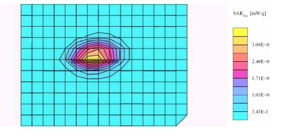
Validation Dipole SAR 1900 MHz (Ambient Temp = 23 C, Liquid Temp = 21 C) SAM Phantom; Flat Section; Position: (90°,90°); Frequency: 1900 MHz Probe: ET3DV6 - SN1604; ConvF(4.90,4.90,4.90); Crest factor: 1.0; Body 1900 MHz:  $\sigma = 1.53$  mho/m  $\epsilon_r = 55.5 \rho = 1.00$  g/cm<sup>3</sup> Cube 5x5x7: SAR (1g): 3.37 mW/g, SAR (10g): 1.83 mW/g, (Worst-case extrapolation) Coarse: Dx = 12.0, Dy = 12.0, Dz = 10.0 Powerdrift: -0.01 dB
