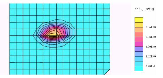
Validation Dipole SAR 1900 MHz (Ambient Temp = 23 C, Liquid Temp = 21 C) SAM Phantom; Flat Section; Position: (90°,90°); Frequency: 1900 MHz Probe: ET3DV6 - SN1604; ConvF(4.90,4.90,4.90); Crest factor: 1.0; Body 1900 MHz:  $\sigma = 1.53$  mho/m  $\epsilon_r = 55.5 \ \rho = 1.00$  g/cm<sup>3</sup> Cube 5x5x7: SAR (1g): 3.37 mW/g, SAR (10g): 1.82 mW/g, (Worst-case extrapolation) Coarse: Dx = 12.0, Dy = 12.0, Dz = 10.0 Powerdrift: -0.01 dB
