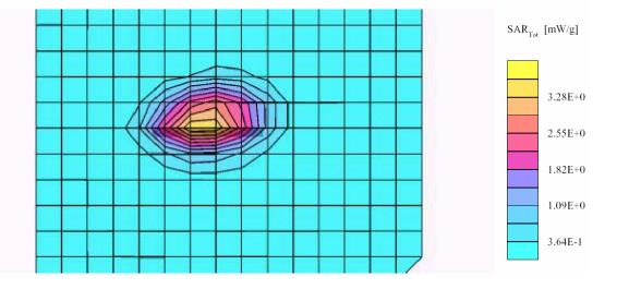
Validation Dipole SAR 1900 MHz (Ambient Temp = 23 C, Liquid Temp = 21 C) SAM Phantom; Flat Section; Position: (90°,90°); Frequency: 1900 MHz Probe: ET3DV6 - SN1604; ConvF(4.90,4.90,4.90); Crest factor: 1.0; Body 1900 MHz:  $\sigma = 1.53$  mho/m  $\epsilon_r = 55.5 \rho = 1.00$  g/cm<sup>3</sup> Cube 5x5x7: SAR (1g): 3.61 mW/g, SAR (10g): 1.95 mW/g, (Worst-case extrapolation) Coarse: Dx = 12.0, Dy = 12.0, Dz = 10.0 Powerdrift: 0.01 dB
