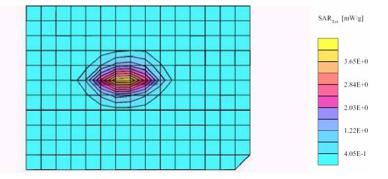
Validation Dipole SAR 1900 MHz (Ambient Temp = 23 C, Liquid Temp = 21 C) SAM Phantom; Flat Section; Position: (90°,90°); Frequency: 1900 MHz Probe: ET3DV6 - SN1604; ConvF(4.90,4.90,4.90); Crest factor: 1.0; Body 1900 MHz:  $\sigma$  = 1.53 mho/m  $\epsilon_r$  = 55.5  $\rho$  = 1.00 g/cm<sup>3</sup> Cube 5x5x7; SAR (1g): 3.77 mW/g, SAR (10g): 2.08 mW/g, (Worst-case extrapolation) Coarse: Dx = 12.0, Dy = 12.0, Dz = 10.0 Powerdrift: -0.05 dB
