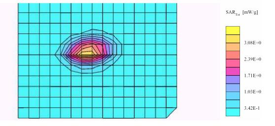
Validation Dipole SAR 1900 MHz (Ambient Temp = 23 C, Liquid Temp = 21 C) SAM Phantom; Flat Section; Position: (90°,90°); Frequency: 1900 MHz Probe: ET3DV6 - SN1604; ConvF(4.90,4.90,4.90); Crest factor: 1.0; Body 1900 MHz:  $\sigma = 1.53$  mho/m  $\epsilon_r = 55.5 \rho = 1.00$  g/cm<sup>3</sup> Cube 5x5x7: SAR (1g): 3.58 mW/g, SAR (10g): 1.94 mW/g, (Worst-case extrapolation) Coarse: Dx = 12.0, Dy = 12.0, Dz = 10.0 Powerdrift: 0.00 dB
