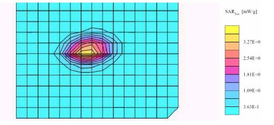
Validation Dipole SAR 1900 MHz (Ambient Temp = 23 C, Liquid Temp = 21 C) SAM Phantom; Flat Section; Position: (90°,90°); Frequency: 1900 MHz Probe: ET3DV6 - SN1604; ConvF(4.90,4.90,4.90); Crest factor: 1.0; Body 1900 MHz:  $\sigma$  = 1.53 mho/m  $\epsilon_r$  = 55.5  $\rho$  = 1.00 g/cm<sup>3</sup> Cube 5x5x7: SAR (1g): 3.63 mW/g, SAR (10g): 1.97 mW/g, (Worst-case extrapolation) Coarse: Dx = 12.0, Dy = 12.0, Dz = 10.0 Powerdrift: 0.01 dB
