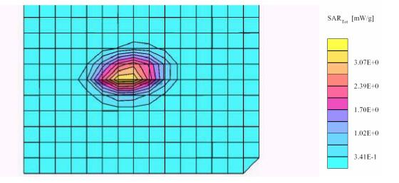
Validation Dipole SAR 1900 MHz (Ambient Temp = 23 C, Liquid Temp = 21 C) SAM Phantom; Flat Section; Position: (90°,90°); Frequency: 1900 MHz Probe: ET3DV6 - SN1604; ConvF(4.90,4.90,4.90); Crest factor: 1.0; Body 1900 MHz:  $\sigma = 1.53$  mho/m  $\epsilon_r = 55.5 \ \rho = 1.00$  g/cm<sup>3</sup> Cube 5x5x7: SAR (1g): 3.60 mW/g, SAR (10g): 1.95 mW/g, (Worst-case extrapolation) Coarse: Dx = 12.0, Dy = 12.0, Dz = 10.0 Powerdrift: 0.00 dB
