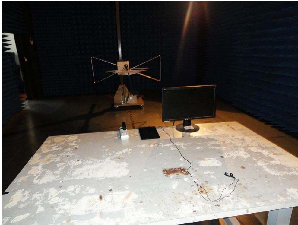
Radiated Emission Test Setup:
