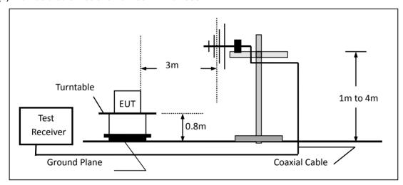
(c) For radiated emissions above 1000MHz
