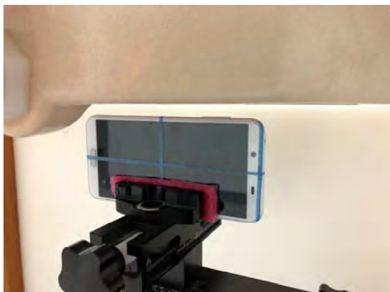
Fig.14 EUT Left side to flat phantom
