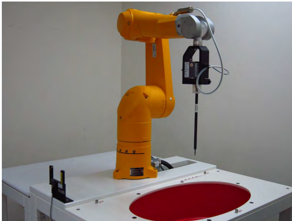
Fig.1 Photograph of the SAR measurement system
