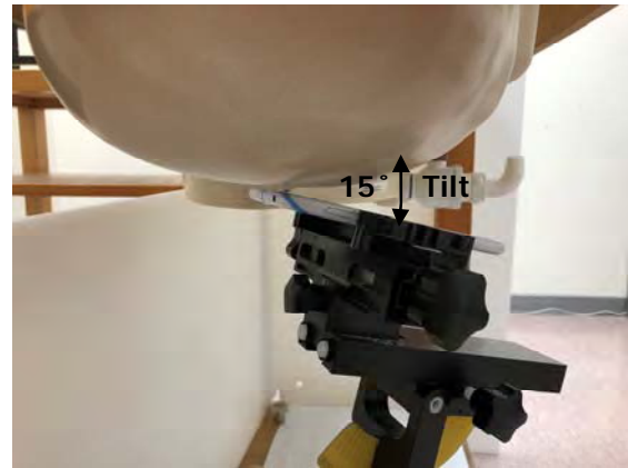
Fig.4 Right Head Section / Ear-Tilt Position(15°)
