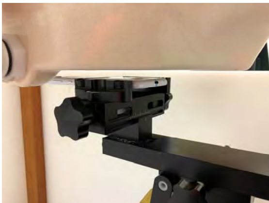
Fig.10 EUT Back side to flat phantom
