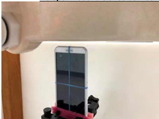
Fig.12 EUT Bottom side to flat phantom
