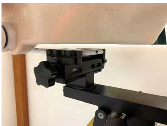
Fig.8 EUT Back side to flat phantom
