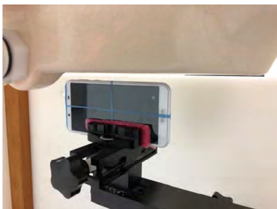
Fig.13 EUT Right side to flat phantom
