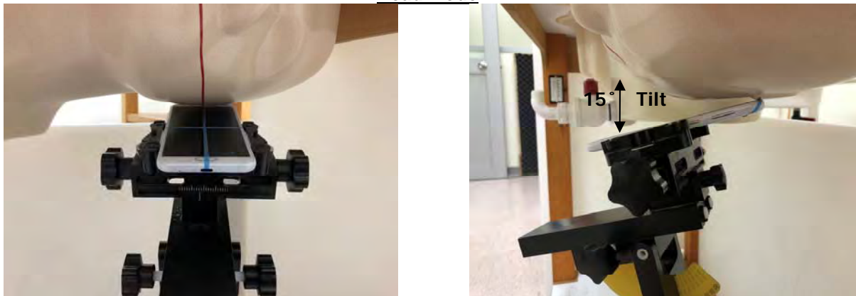
Fig.6 Left Head Section / Ear-Tilt Position(15°)
