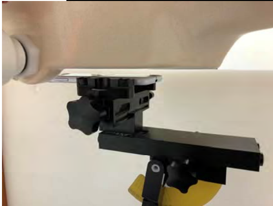
Fig.9 EUT Front side to flat phantom
