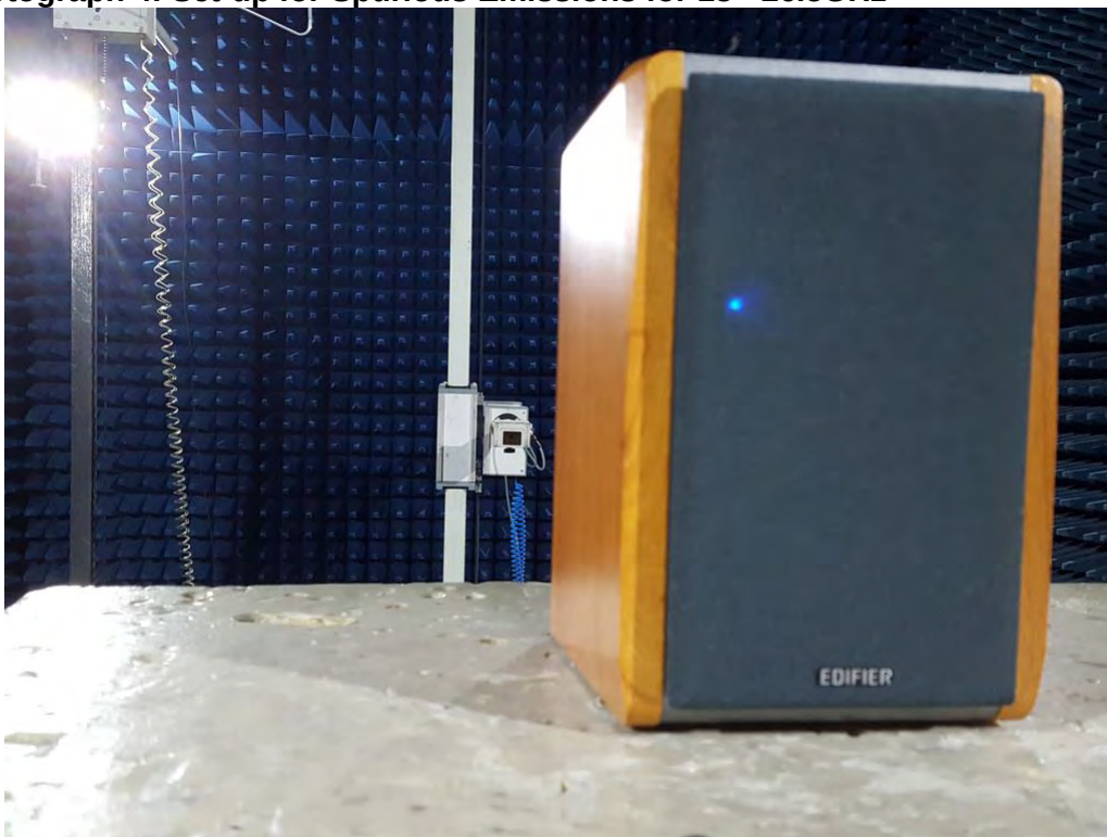
Photograph 4: Set-up for Spurious Emissions for 18 - 26.5GHz
